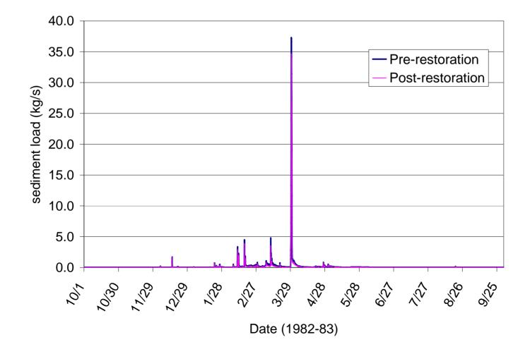
Comparison of monthly sediment load at Doyle Crossing between the pre-restoration and post-restoration conditions (Oct.1982 - Sep.1983)
