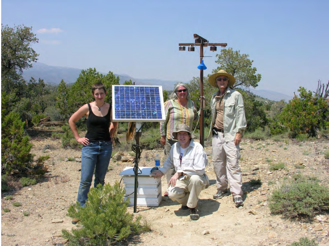
Figure 3: Air pollution monitoring site with active ozone instrument and passive samplers in the White Mountains during 2007. Research was conducted by collaborators from the USDA Forest Service Pacific Southwest Research Station, University of California, and the Saint Mary’s College. Photo credit Andrzej Bytnerowicz.
